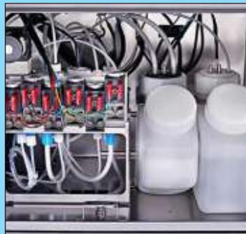
Single print head and recovery diaphragm pump design make more stable and durable. Double mixing design prevent the ink precipitation.
